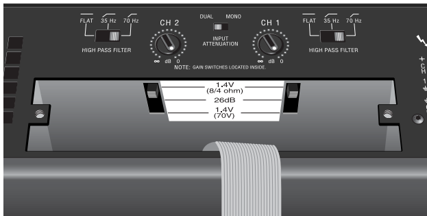
Figure 5.1 Input Sensitivity Switches for CTs 600/1200
