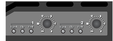
Figure 5.7 Tamper-Resistant Hole Plugs Installed in a CE 2000TX Amplifier
