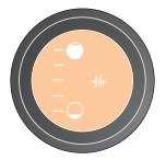
The lighted bar shows how much charge is left in your battery. A flashing light will warn you that the battery is getting low. Two flashing lights mean you must have the battery changed or recharged.
