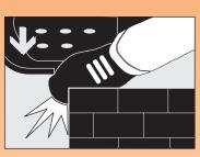
A foot or hand caught between the truck and a wall, post or any fixed object will be crushed or even cut off.
