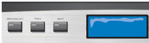
Figure 4.3 LCD Control Screen and Its Controls. Left-to-right: Menu/Select Button, Prev Button, Next Button, LCD Control Screen
