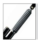
ELECTRIC LIFT CYLINDER Useful all year long. It raises the deck or snow blade easily.
