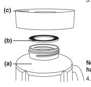
3. Turn the locking ring with cutting assembly (c) upside down, and place the blade end in the blender jar opening. Engage threads by twisting the locking ring clockwise until tightened. Make sure locking ring is tightly fastened to blender jar. Once assembled, turn the blender jar right-side up.
