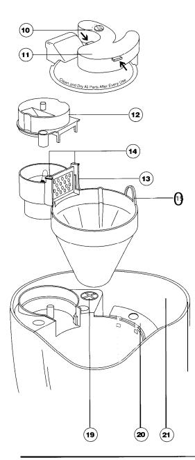
11. Filter Basket Cover/Filter Holder: To put on or remove, grasp in area as indicated by arrows. NOTE: COVER MUST BE IN PLACE FOR UNIT TO OPERATE. Cover becomes hot after coffee is brewed. Use caution when removing cover.
