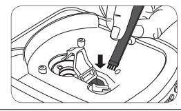
Open grind chute lever to allow grounds into filter basket.
