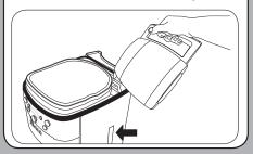
Open the filter basket door by pressing the Release button and insert a paper filter or permanent filter into the filter basket holder. Replace the cover, line up arrows, and close door.
