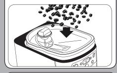
Select the amount of beans you wish to grind with the Grind Control knob. Select your desired coffee strength with the Strength Control button. Your selected coffee strength will be indicated on the LCD display.
