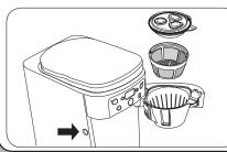
Remove hopper lid, fill with beans, and replace the lid.
