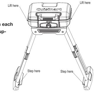
Step 4: While holding grill off the ground, swing the legs apart and lower the grill slowly at the same time, continue until grill is flat on the ground with legs to the sides
