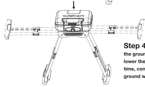
Step 5: Push legs inward toward grill chassis. You must push the leg release button (as shown) to collapse legs under grill
