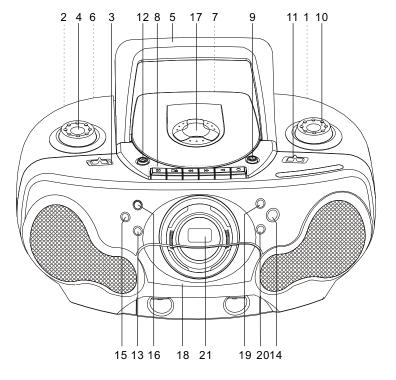
2. Stereo Headphone Jack 3. POWER Switch (ON/OFF) 4. VOLUME Control 5. Carrying Handle 6. AC Socket (Rear of Unit) 7. Battery Compartment (Rear of Unit) 8. Cassette Buttons : PAUSE (III) STOP/EJECT (■▲) FAST FORWARD (++)
