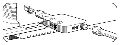
If your antenna system has two sets of twin 300-ohm leads, you must obtain a combiner (available at your local electronics store). Place one set of twin leads underneath the screws on the combiner and tighten the screws. Do the same with the other set of twin leads. Press the cable from the combiner onto the antenna terminal on the back of your TV/VCR Combination.
