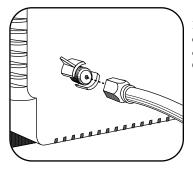
If your cable system does not require the use of a cable box, simply press or screw the incoming cable onto the antenna terminal on the back your TV/VCR Combination.
