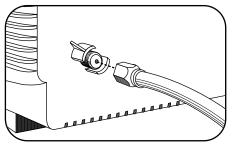
If your antenna ends in a single coaxial lead, simply press or screw the cable onto the antenna terminal on the back of your TV/VCR Combination.
