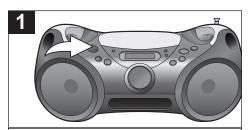
Rotate the Function control to the AM or FM ST position to turn the unit on and select AM or FM ST (Stereo); the band and the frequency will appear in the display.
