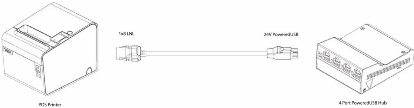
Figure 2-14. Cable, +24V PoweredUSB to 1x8 PoweredUSB
