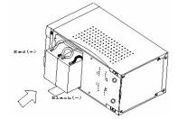
Install the replacement battery by connecting the red wire to the positive (+) terminal of the battery and connecting the black wire to the negative (-) terminal of the battery.
