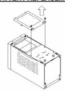
Remove the 2 retaining screws then push the battery cover backward and remove the cover.
