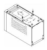
4. Slide the battery back into the compartment. Turn the UPS upside down to help the batteries entirely slide into the compartment. Replace the cover and the retaining screws.
