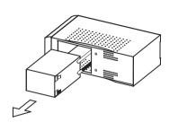
2. Lean the UPS to one side and pull out the battery partially from the compartment. Disconnect the battery wires from the battery, and then remove the battery from the compartment.
