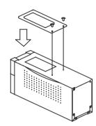
4. Slide the battery back into the compartment. Turn the UPS upside down to help the batteries entirely slide into the compartment. Replace the cover and the retaining screws.
