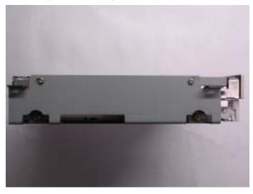
Step 3: Fasten the transferring bar with a pair of screws on the back of the CD-ROM.
