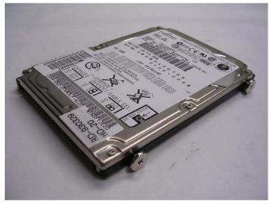
Step 2: Cover the screws with four pieces of anti-vibration rubber
