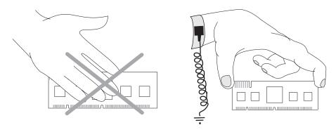
Confirm that the wrist-strap is grounded. Remove the modem board from its anti-static packaging, being careful to not touch the components or metal parts of the board (see the figure).
