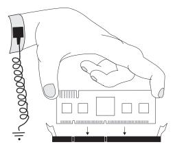
Insert the board carefully into the slot, aligning the indentations in the board with the guides of the slot. Forcing the board or pushing it in at an angle can damage the board and the slot.
