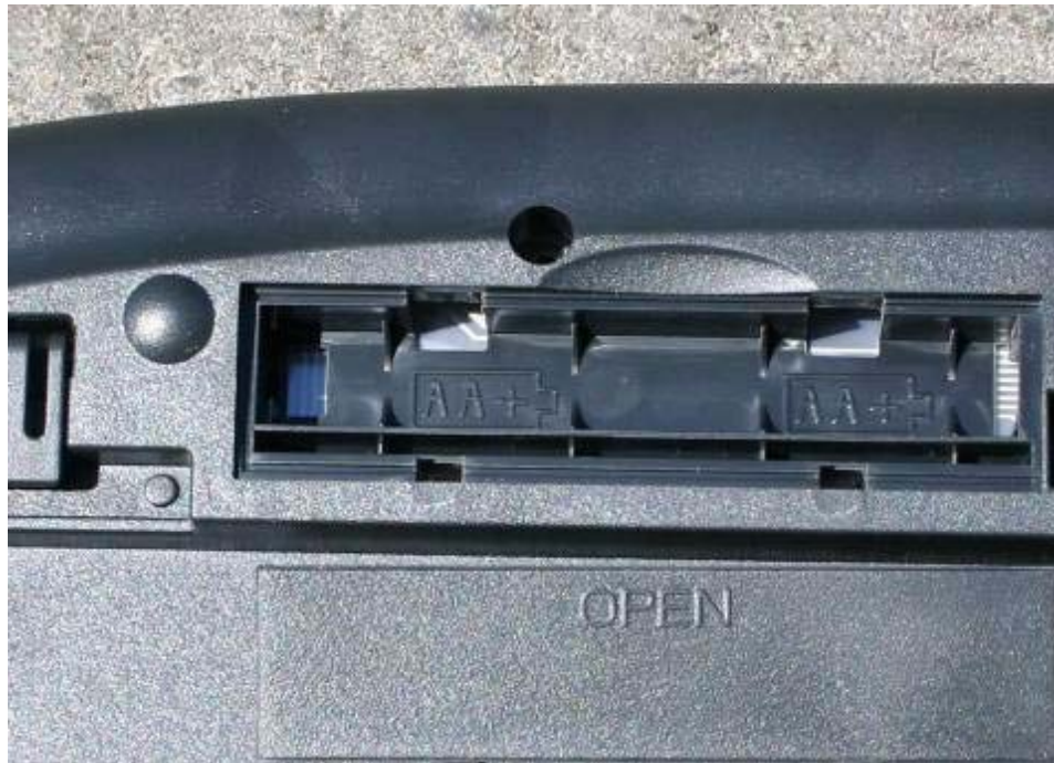
Figure 4-4 shows the integrated battery compartment located on the bottom side of the keyboard. The battery compartment cover is also shown.
