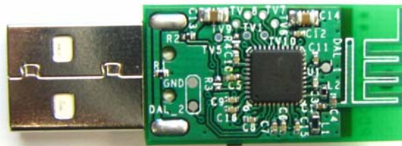
Figure 5-2. RDK Bridge Bottom
