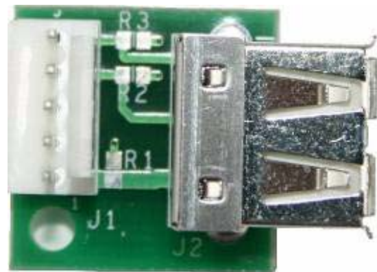
Figure 5-3. Cypress USB Programming Adapter
