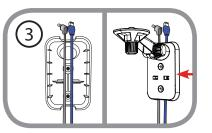
Fasten the mounting bracket to the wall using the screws provided.
