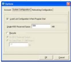
In order to allow old video files to be overwritten and replaced by new recorded files, place a check mark in the **Recycle** Box and click on **By HDD Reserved Space** or **By Time**. The **Single HDD Reserved Space** field refers to the amount of space left on your drive before overwrite takes place. For instance if you enter 1000 MB, and your total hard drive space is 3000 MB, as soon as your drive reaches 2000 MB capacity, your files will be
