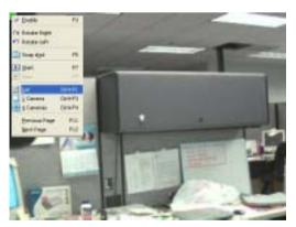
These features will be available: Enable, Rotate Right, Rotate Left, Snap Shot, Start, Stop, List, 1 Camera or 4 Cameras, Previous Page and Next Page.
