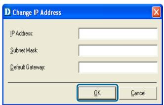
Enter the new IP Address, the Subnet Mask and the Default gateway into the respective fields and click OK. IPView Lite will apply the new IP Address to the camera.
