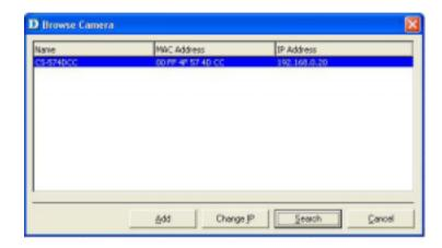
Highlight the camera you wish to add and click on **Add**. The **Add Camera** dialog box will appear once again with the IP Address entered. Click on **Add**. The camera will automatically be added into the IPView Lite list view.
