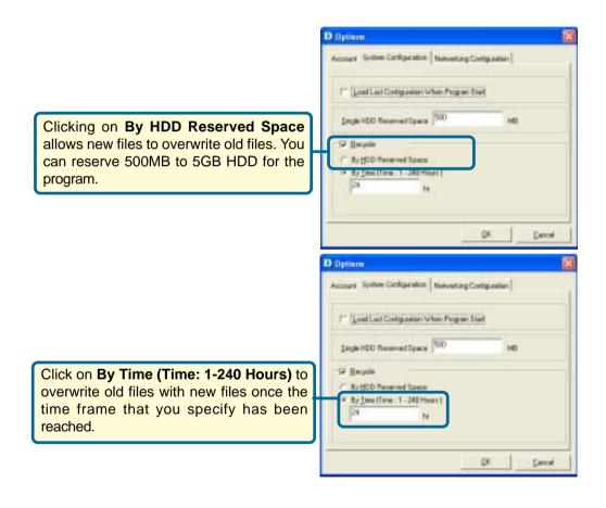
Note: Selecting the **Recycle** option will disable the **Recording File Path Settings** in the **Recording** menu.
