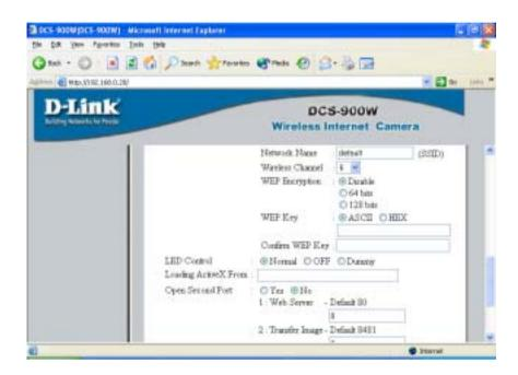
To enable WEP Encryption, first decide which WEP key format will be applied. Click on the ASCII or HEX check box to select the type of format, then input the WEP key. To Confirm the WEP key you must enter the data once again in the Confirm WEP Key field.
