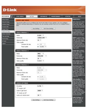
**Fixed quality:** Select the image quality level for the camera to try to maintain. High quality levels will result in increased bit rates.
