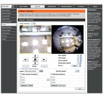
Preset List: To add a preset to the sequence, select it from the dropdown box at the bottom of this window, set the Dwell time to determine how long the camera view will stay at that preset, then click the Add button. The preset name will appear in the list, followed by the dwell time to view that preset for.
