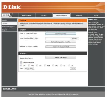
**Save To Local** Click the **Save Configuration** button to save the current camera configuration **Hard Drive:** to your local PC.
