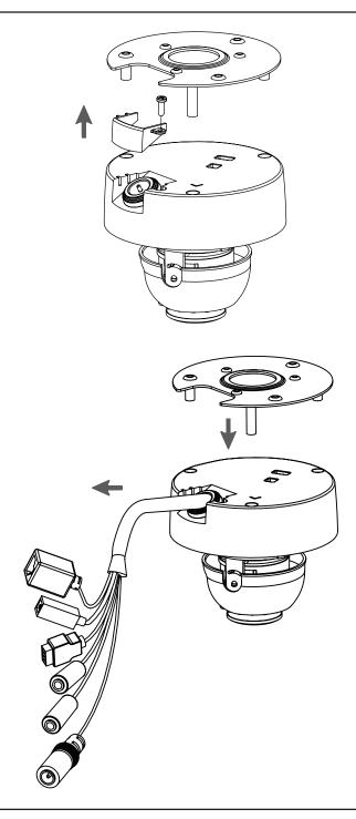
Reattach the top part of the camera housing, and secure it by tightening the three retaining screws.
