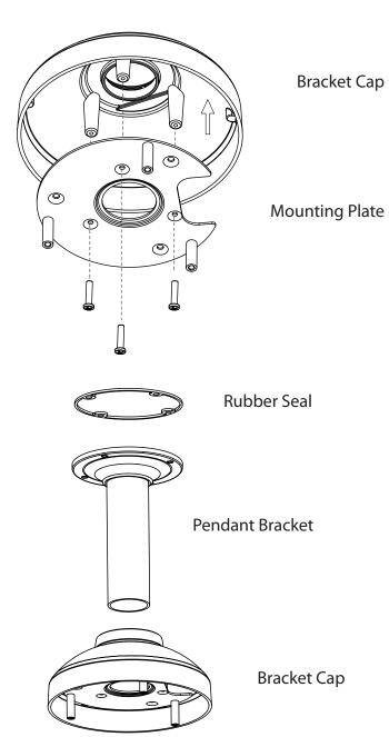
Begin the process of reattaching the bottom part of the camera housing, by first pushing the cable sheath up through the pendant mount. Once the cable has been pushed through, you can then firmly reattach the bottom part of the camera housing, and secure it by tightening the three retaining screws.
