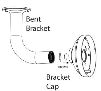
Begin the process of reattaching the bottom part of the camera housing, by first pushing the cable sheath up through the bent mount. Once the cable has been pushed through, you can then firmly reattach the bottom part of the camera housing, and secure it by tightening the three retaining screws.
