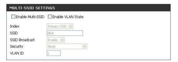
**Index:** The Primary SSID and Security cannot be changed here .Those values follow the setting in SETUP>WIRELESS.
