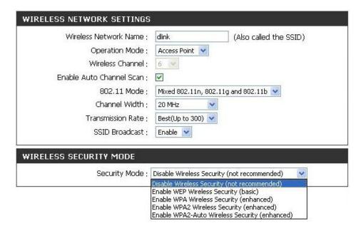
802.11 Mode: Select the appropriate 802.11 mode based on the wireless clients in your network. The drop-down menu options are 802.11g Only, Mixed 802.11b/g, 802.11b Only, 802.11n Only, or Mixed 802.11b/g/n.
