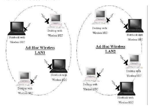
An Ad-Hoc wireless LAN is a group of computers, each equipped with one wireless adapter, connected as an independent wireless LAN. Computers in a specific Ad-Hoc wireless LAN must be configured at the same radio channel.
