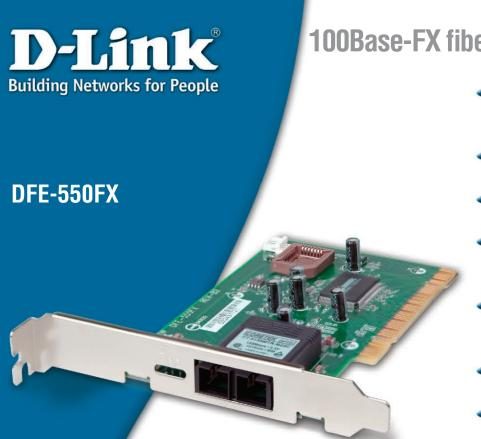
100Base-FX fiber based Network Adapter
