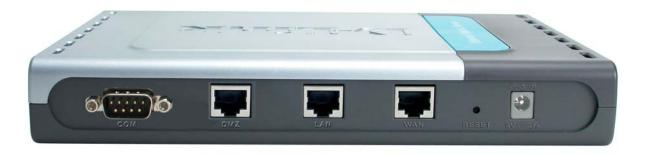
Console: Serial access to the firewall software, 9600, 8bit, None Parity, 1Stop bit.
