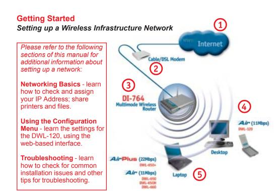
Please remember that **D-Link Air** wireless devices are pre-configured to connect together, right out of the box, with their default settings.
