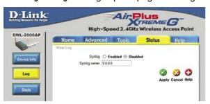
When you click on **Log Settings** in the previous window, the window at left appears. Select **Enabled** to save the log. In the **Syslog Server** field, input the IP Address of the computer on the network to which you wish to save the log settings. Click **Apply** to save the changes.
