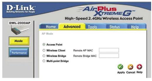
The DWL-2000AP can be configured to perform in any of four modes: a Wireless Access Point; a Wireless Client; a Wireless Bridge; or a Multi-Point Bridge.
