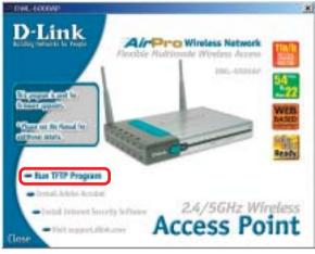
\*To run the **D-Link TFTP program**, insert the DWL-6000AP CD-ROM, and click on **Run TFTP Program**. Or go to Start > Run > and type **d:\tftpd.exe** (where "d:\" refers to the CD-ROM drive on the computer.) (Note: The TFTP program must be running to upload the firmware.)
