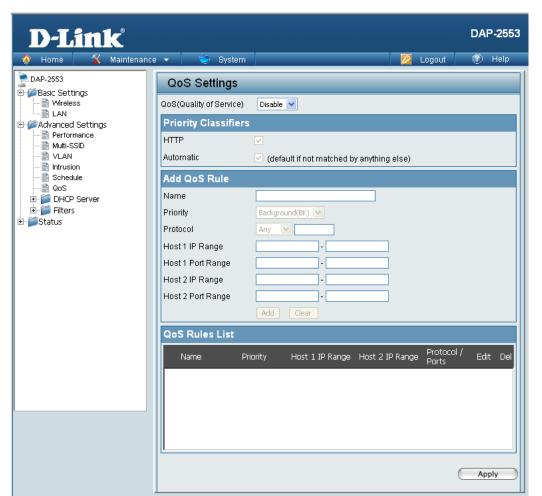
Automatic: When enabled, this option causes the access point to automatically attempt to prioritize traffic streams that it doesn't otherwise recognize, based on the behavior that the streams exhibit. This acts to de-prioritize streams that exhibit bulk transfer characteristics, such as file transfers, while leaving interactive traffic, such as gaming or VoIP, running at a normal priority.
