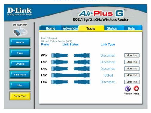
The above window is a Virtual Cable Tester and it shows the user the current status of the ports of the Router. In this window, we can see that LAN 3 port is connected at a speed of 100Mbps Full (duplex) and all the other connections do not have a valid link. Clicking the **More Info** button will open an additional window with more information about this connection, as shown below.
