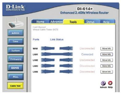
Diagnostic Cable Tester is an advanced feature that integrates a LAN cable tester on every Ethernet port on the router. Through the graphical user interface (GUI), Cable Tester can be used to remotely diagnose and report cable faults such as opens, shorts, swaps, and impedance mismatch. The Cable Tester feature significantly reduces service calls and returns by allowing users to easily troubleshoot their cable connections.
