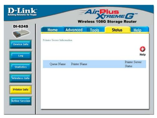
The **Printer Info** window displays a list of Printers that are using the DI-624S as a print server. These printers are defined by their **Queue Name** and **Printer Name**. The status of these printers is located to the right under the heading **Printer Server Status**.
