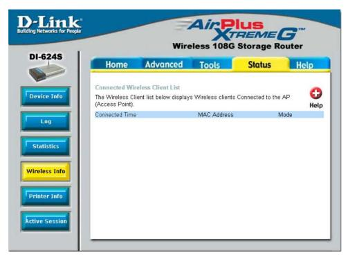
The wireless client table displays a list of current connected wireless clients. This table also displays the MAC address and mode of the connected wireless client.
