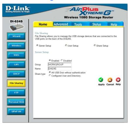
To set up the DI-624S as a file server, the user needs to configure four parts associated with this window. Each part has a corresponding radio button and when clicked, will open up to a new window to configure.
