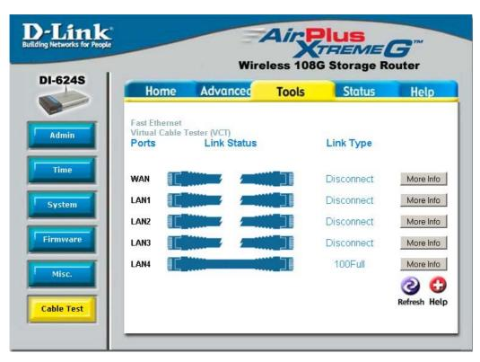
The above window is a **Vitrual Cable Tester** and it shows the user the current status of the ports of the Router. In this window, we can see that LAN4 port is connected at a speed of 100Mbps Full (duplex) and all the other connections do not have a valid link. Clicking the **More** Info button will open an additional window with more information about this connection, as shown below.
