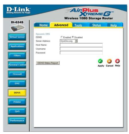
Note: DDNS requires that an account be setup with one of the supported DDNS servers prior to engaging it on the router. This function will not work without an accepted account with a DDNS server.
