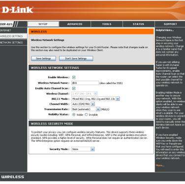
Visibility Status: Select Invisible if you do not want the SSID of your wireless network to be broadcasted by the DIR-625. If Invisible is selected, the SSID of the DIR-625 will not be seen by Site Survey utilities so your wireless clients will have to know the SSID of your DIR-625 in order to connect to it.
