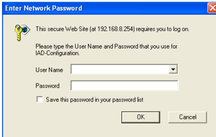
DVG-5112S does not allow multiple people to configure the gateway simultaneously. Please remember to logout or restart the system if you are not using the web configuration function.
