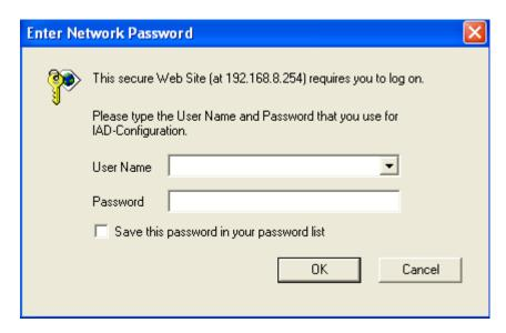
The gateway doesn't allow multiple people to configure the gateway at same time. If a user logs into the system, other users from different IP addresses cannot login at the same time. Please remember to logout or restart the system if not using the web configuration function.
