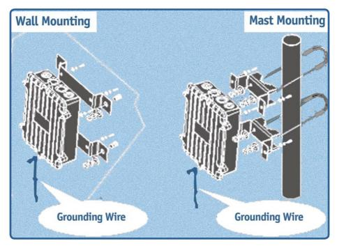
The DWL-1750 can be mounted on the side of a building or mounted to a mast as shown above. A wall mount is a convenient location if the roof overhang is not excessive and/or the location is high enough to provide a clear line of sight.
