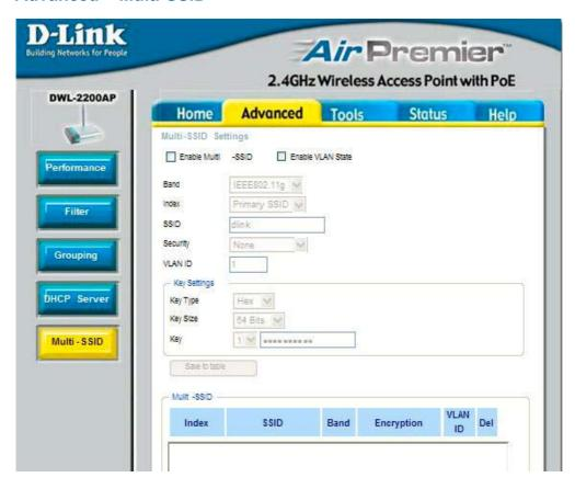
If you want to configure the Guest and Internal networks on Virtual LAN (VLANs), the switch and DHCP server you are using must suppport VLANs. As a prerequisite step, configure a port on the switch for handling VLAN tagged packets as described in the IEEE802.1Q standard.
