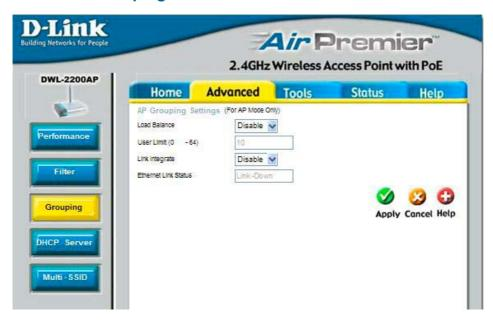
The D-Link DWL-2200AP allows you to balance the distribution of wireless client connections across multiple access points. Using load balancing, you can prevent scenarios where a single access point in your network shows performance degradation because it is handling a disproportionate share of the wireless traffic.
