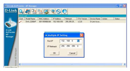
Select the AP that you want to assign an IP address to and click the IP button. Enter the IP address and IP netmask for the selected device and click OK.
