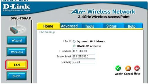
**Dynamic IP Address:** Select this option if you would like to have an IP address automatically assigned to the DWL-700AP by a DHCP server in your network.
