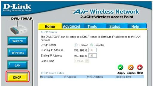
**DHCP Server:** Select **Enabled** or **Disabled**. Disabled is the default setting. If you want to use the access point as a DHCP server to automatically assign dynamic IP addresses on the network, you will select Enabled.
