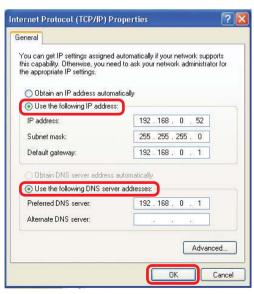
You have completed the assignment of a static IP address. (You do not need to assign a static IP address if you have a DHCP-capable gateway/router.) 32
