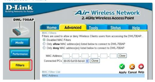
Use MAC Filters to allow or deny computers by their MAC Addresses from accessing the DWL-700AP. You can either manually add a MAC Address or select the MAC Address from the list of clients that are currently connected to the broadband router (Connected PCs). The default setting is Disabled MAC Filters.
