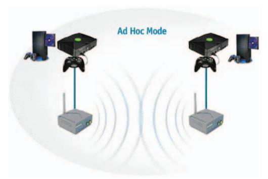
This example illustrates an **Ad-Hoc** setup. Simply connect the DWL-G810 (*refer to the Quick Installation Guide*) to your Ethernet-capable network device (*in this case, a gaming console*) and you will be able to connect wirelessly with other gaming consoles also connected to DWL-G810's.
