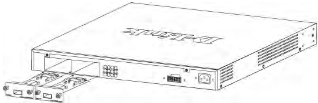
Figure 23. Inserting the optional module into the Switch (DWS-3026)
