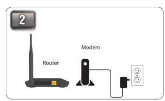
Position your router close to your modem and a computer. Place the router in an open area of your intended work area for better wireless coverage.
