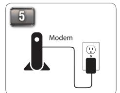
Reconnect the power adapter to your cable or DSL broadband modem and wait for two minutes.
