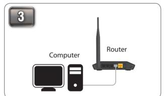
If you are currently using a router, disconnect all the cables connected to it before installing the DIR-605L. Unplug the Ethernet cable from your modem that is connected to your computer. Plug it into the LAN port labeled 1 on the back of your router. The router is now connected to your computer.
