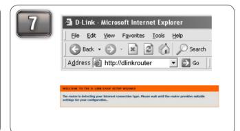
From the computer you connected the router to, open a web browser and enter http://192.168.0.1 or http://dlinkrouter. Press Enter and you will be directed to the D-Link Setup Wizard page, which will detect your Internet connection type. Follow the on-screen instructions to configure your Internet settings. After setting up your router, you will be given the option to create a mydlink account. Go to www. mydlink.com and enter your acount information.
