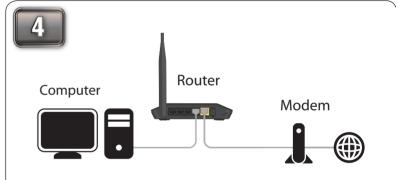
Plug one end of the included blue Ethernet cable that came with your router into the yellow port labeled **INTERNET** on the back of the router. Plug the other end of this cable into the Ethernet port on your modem.
