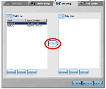
**Step 5)** Once you have added the INTERNAL site as described in Step 3 and 4, your INTERNAL site will be added to the sites list as shown in the screenshot below (circled in red). Select the INTERNAL site from the drop down list, and then Click the CONNECT button as shown to the left of the drop down list.
