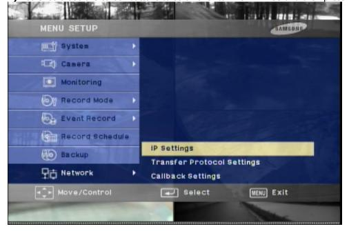
**5)** Now that you are in the IP SETTINGS setup menu as shown below, we need to edit the network settings to match your router. Use the cursor buttons and enter button to scroll down, select and change the IP address, and then adjust the gateway and DNS. Ding this will make sure your DVR's Network and IP settings are setup to work with your router. The important settings are listed below:
