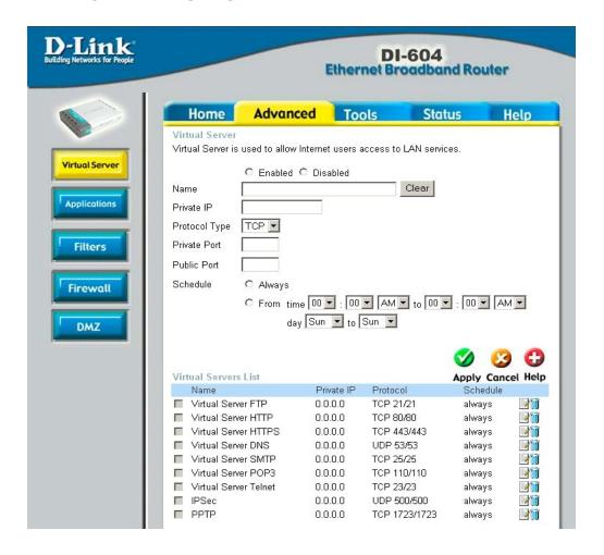
The VDI-604 can be configured as a virtual server so that remote users accessing Web or FTP services via the public IP address can be automatically redirected to local servers in the LAN network.
