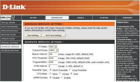
Fragmentation: The fragmentation threshold, which is specified in bytes, determines whether packets will be fragmented. Packets exceeding the 2346 byte setting will be fragmented before transmission. 2346 is the default setting.
