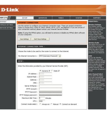
**PPTP:** Select **Dynamic** (most common) or **Static**. Select **Static** if your ISP assigned you the IP address, subnet mask, gateway, and DNS server addresses.
