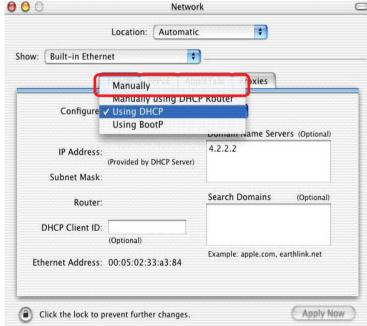
The default IP address of the Print Server is 192.168.0.10. Manually change your IP Address to 192.168.0.x, where x is any number between 1 and 254 (except 10 which is the IP Address of the Print Server.) The IP Addresses and Subnet Mask shown here are examples only.
