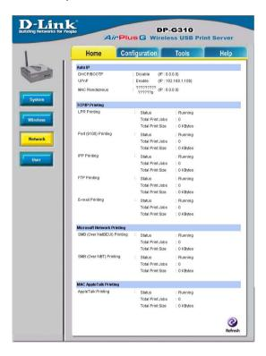
**Auto IP:** This field contains the current settings of TCP/IP, including DHCP/BOOTP, UPnP, and MAC Rendezvous. The items in this field are configured in **Configuration>Network>TCP/IP**.
