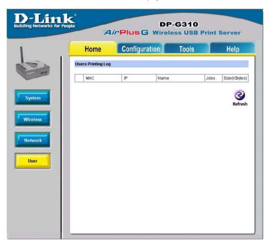
**Users Printing Log:** The items in this field display the user(s) information, which include the user(s) Mac address, IP address, name, and status of printing tasks.
