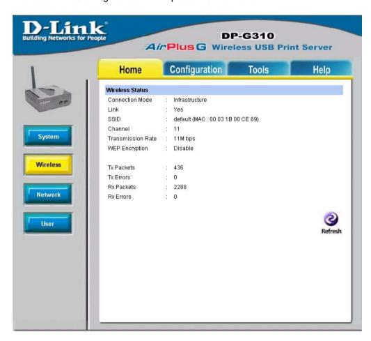
**Wireless Status:** The items in this field display information about the wireless LAN, such as the connection mode (Infrastructure or Ad-Hoc), SSID, channel, data transfer rate, WEP encryption, and the packets status.
