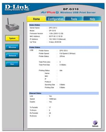
**Device Status:** Information about the print server, including the firmware version, MAC/IP address, and the "up time" can be found in this field.
