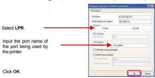
Additional Port Information Required The device could not be identified.
