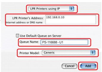
In the **Queue Name** field, type in the **Port Name** of the PostScript printer that is connected to the Print Server. The **Port Name** illustrated here is only an example. Select the printer model from the dialog box.
