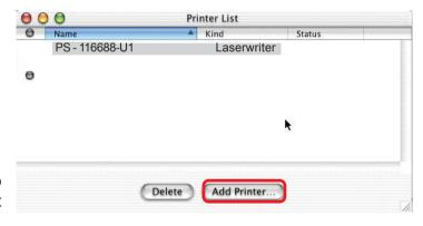
Then select the printer model from the dialog box displayed here. Click **Add Printer** and the Printer Port configuration is complete. Select the Printer Port just configured in the Print window. Click **Print** to print your document.
