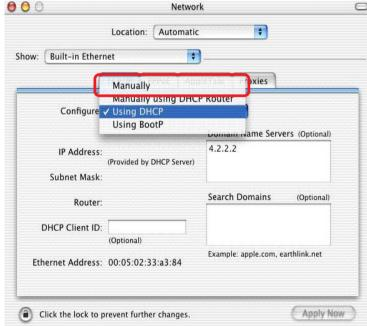
The default IP address of the Print Server is 192.168.0.10. Manually change your IP Address to 102.168.0.x, where x is any number between 1 and 254 (except 10 which is the IP Address of the Print Server.) The IP Addresses and Subnet Mask shown here are examples only.
