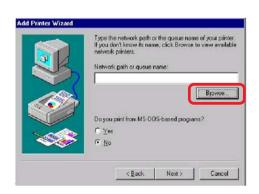
At the next screen, browse for the printer port. Highlight the port as shown. (The **Port Name** in this window is just an example.)
