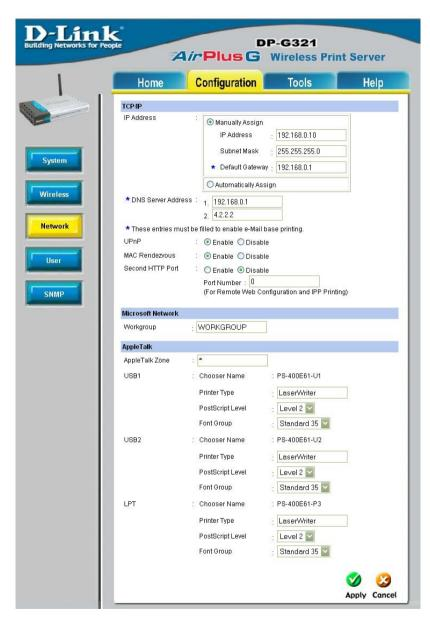
When you select **TCP/IP Protocol** at the **Network** window, the screen below appears. (We recommend that you keep the default settings as shown.) If you need to make changes, make sure to click **Apply** after you have made the changes. (You may wish to make a note of the IP Address.)
