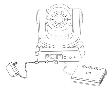
Note: Once power has been established, the Power LED will turn red. When the device has obtained an IP address and is accessible, the Link LED will turn green.
